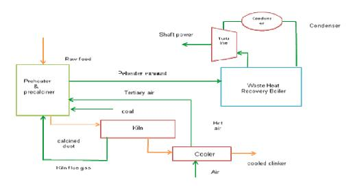
Figure 3: Waste Heat Recovery System
