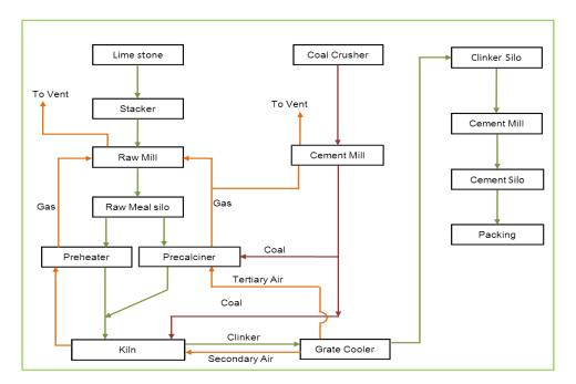
Figure 1: Process Flow Diagram of the Cement Plant
